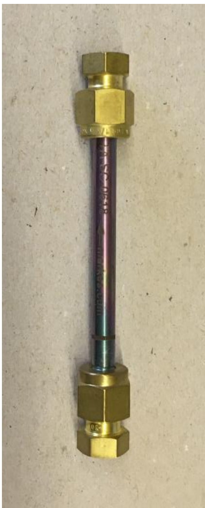
Drawing the smell of mink through this tube traps molecules of the volatile compounds that make it so, um, memorable.
